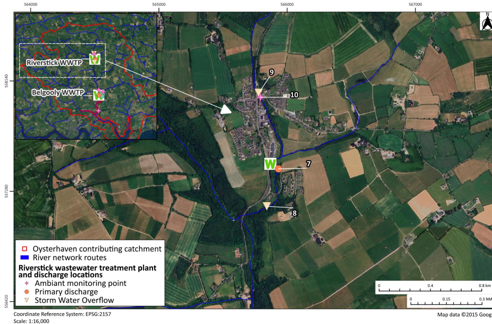
Figure 7-6: Locations of wastewater treatment plants (WWTPs) in Oysterhaven contributing catchment shown in insert on left. In main map, the discharge locations of the Riverstick WWTP in Oysterhaven contributing catchment are displayed. Map IDs cross-referenced to Table 7.3. This figure contains Irish Public Sector Data (EPA) licensed under a Creative Commons Attribution 4.0 International (CC BY 4.0) licence.
